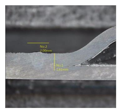
In these materials, DBL technology can achieve stable welding of cooling plate seams at feed rates of 30 m/min. The DBL achieved 30meter-long weld seams with consistent geometry on each plate.
