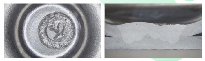
Figure 4: Some designs included large area welds, which caused hot cracks. By using complex beam shapes, DBL technology was able to prevent these defects.
